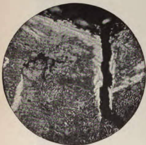
FIG. 5.—BLISTER STEEL. The line of fracture follows the membranes of cementite surrounding the grains.
